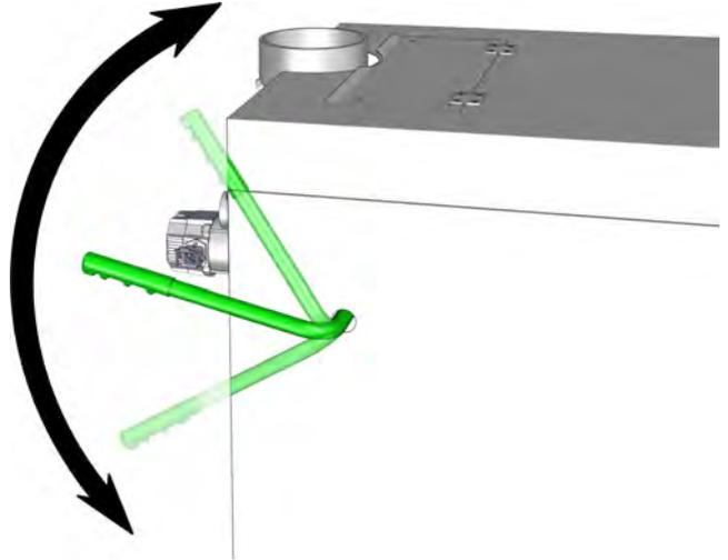
**i** Afterwards, leave the lever pointing towards the rear of the boiler. Then the turbulators remain in position in the water-cooled heat exchanger.
