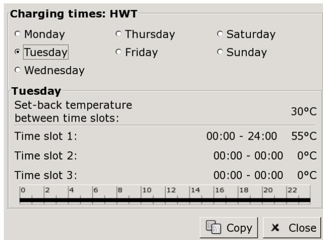
Fig. 10-22: Overview screen for hot water charging times
