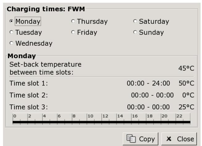
Fig. 10-28: Overview screen for hot water charging times
