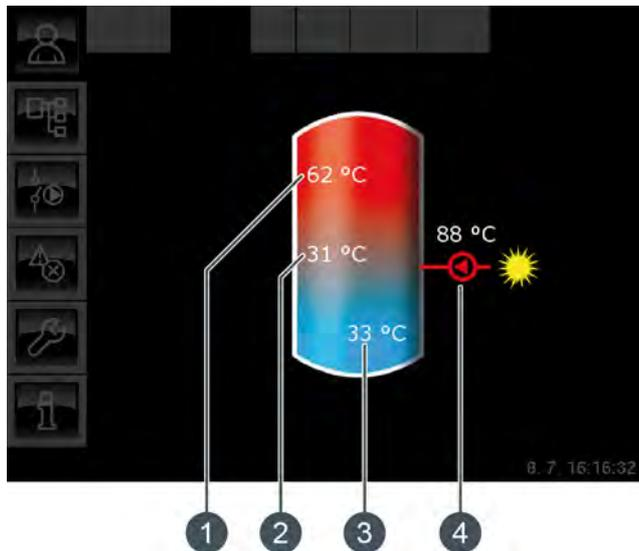
Fig. 10-4: Buffer with solar heating system
