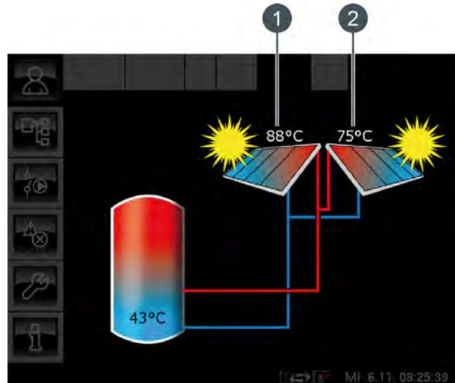
Fig. 10-40: Solar heating system with two solar panels
