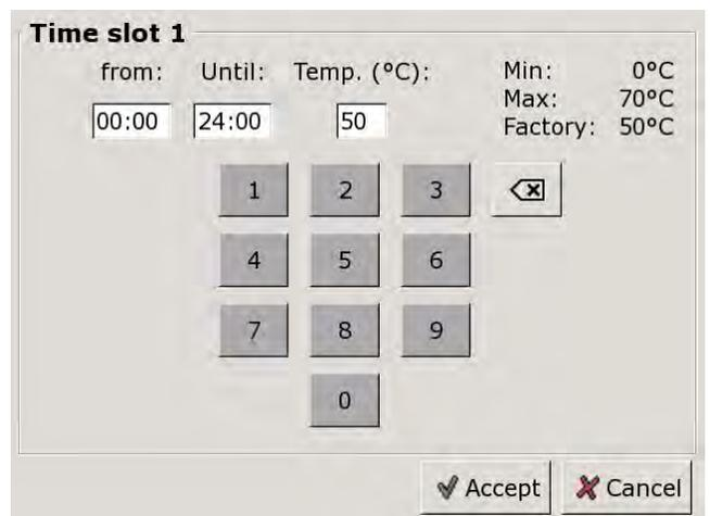
Fig. 10-29: Setting the time slot and hot water temperature
