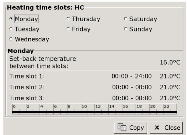
Fig. 10-18: Overview of heating times if a room sensor is installed
