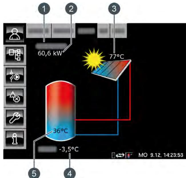
Fig. 10-34: Solar heating system with one tank
