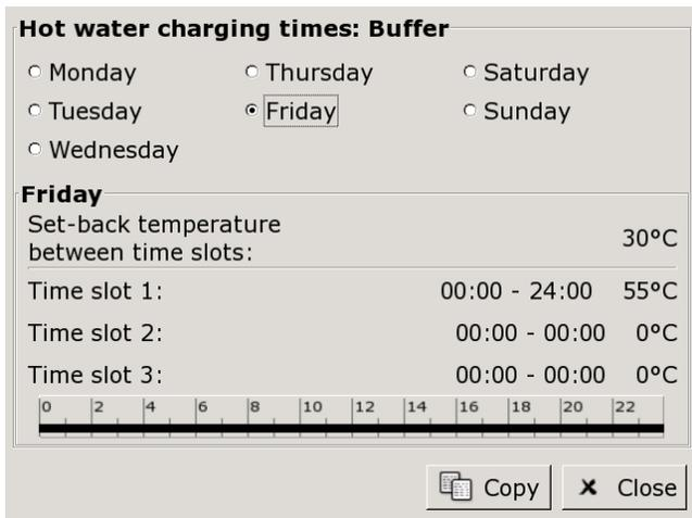
Fig. 10-7: Overview screen for hot water charging times
