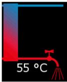
The tap symbol next to the heat exchanger is only displayed if the fresh water module is feeding hot water into the water mains. The temperature shown next to this is the temperature of the hot water currently being supplied.
