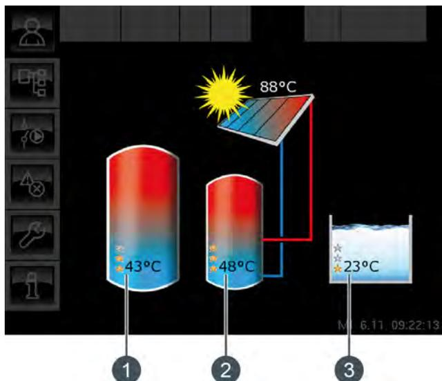
Fig. 10-36: Solar heating system with 3 tanks
