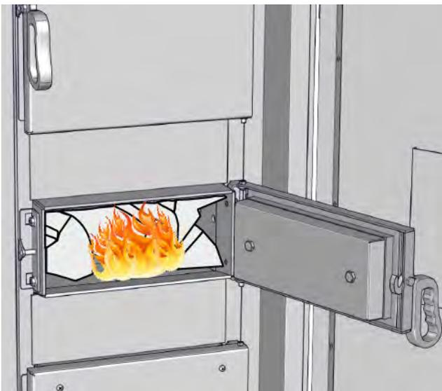
**At 100°C exhaust temperature, close ignition door and insulating door**
