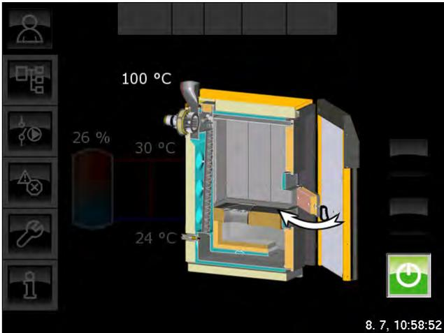
Fig. 10-2: Close ignition and insulation doors
