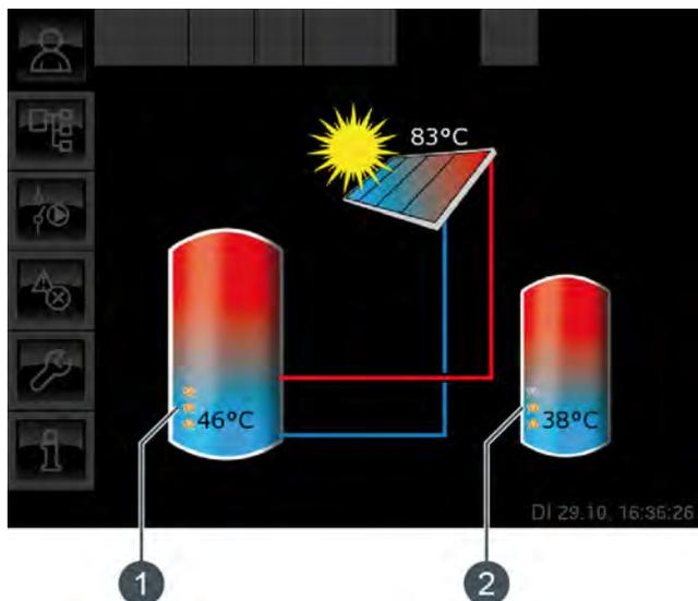
Fig. 10-35: Solar heating system with 2 tanks
