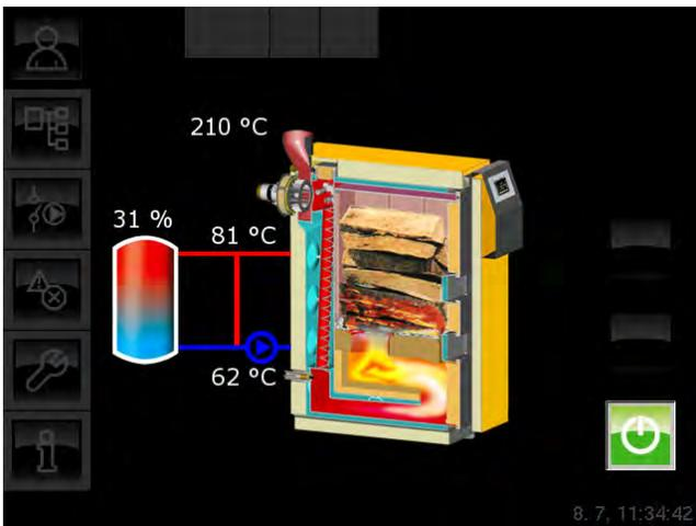
Fig. 10-3: Log boiler in heating mode
