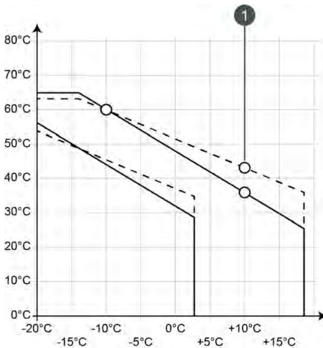
Fig. 10-16: Adjusting the heating curve in the transitional period
