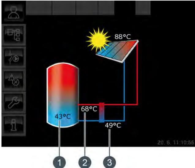
Fig. 10-38: Solar heating system with external heat exchanger
