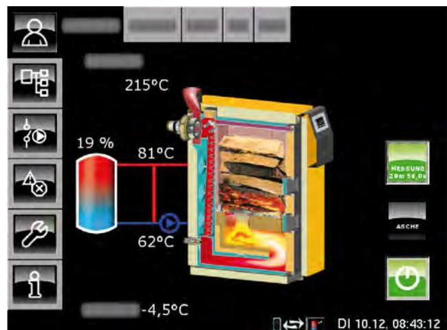
The boiler now runs for 30 minutes at full load. The control system ensures that sufficient heat is channelled to the heating circuits and the hot water tank.
