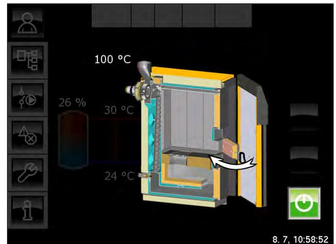
When the insulating door is closed, the boiler automatically switches to [Ignition] mode and, once the residual oxygen content is below 15%, to [Heating] mode. The boiler is now in heating mode and regulates the combustion of the wood independently.
