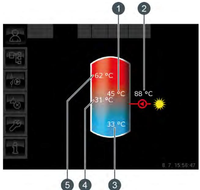
Fig. 10-5: Buffer with solar heating system and stratified charging valve
