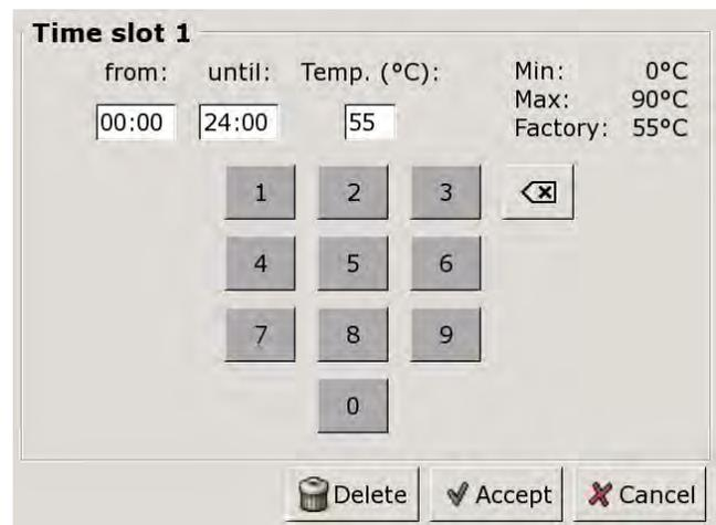
Fig. 10-23: Setting the time slot and hot water temperature
