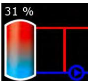
This symbol is displayed next to the boiler as soon as it supplies heat to the buffer. The percent display shows the current buffer charging status.
