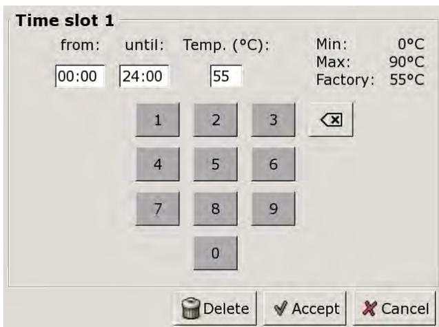
Fig. 10-8: Setting the time slot and hot water temperature
