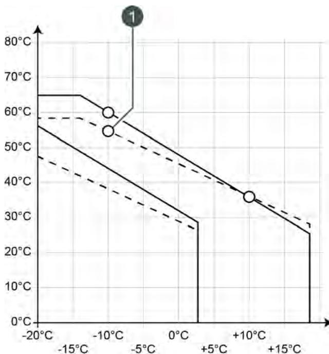
Fig. 10-17: Adjusting the heating curve in the winter
