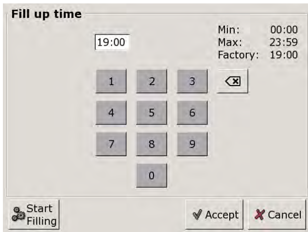
Fig. 7-5: Setting the fill-up time
